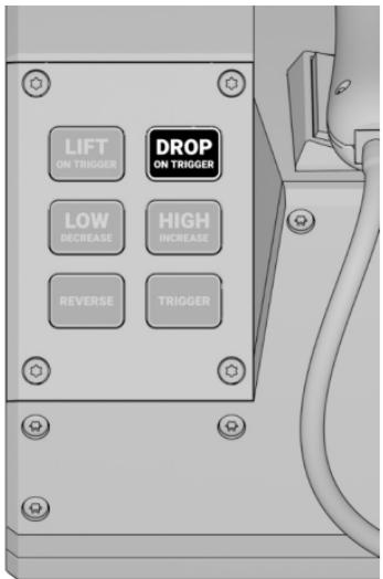
To activate drop mode, press the "Drop" button once to select and arm it. Pressing the button again will start the pump, allowing you to pick up a part.
