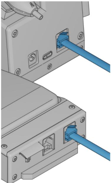
Connect the foot pedal to the Pixel Pump with the included RJ11 cable.
