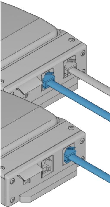
If you have a second foot pedal connect it to the remaining port of the first foot pedal.
